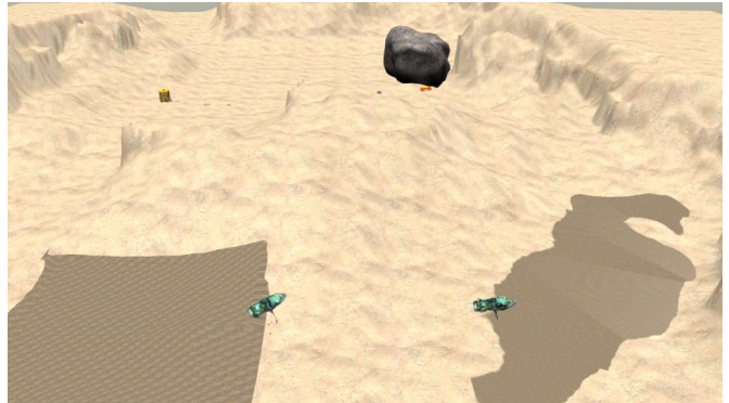
Fig. 8: Integrated scenario with electrical flying lead and bimanual manipulation (top left), surface occlusion (shaded areas at the bottom), and distorted objects (scattered).
